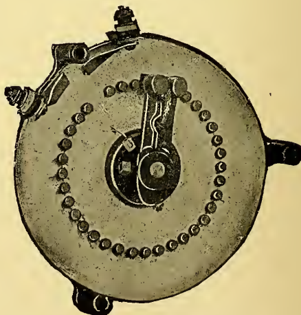
FIG. 241.—The resistance wires of the rheostat are completely enclosed in a vitreous enamel, as can be seen from this reverse view of the rheostat shown in Fig. 240; the contact buttons project through the enamel, are ground off smooth, and thus serve to permit connection of the wire with the sliding shoe.
